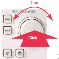
Simply select the desired menu with the spinwheel and click the button to open the submenu.
